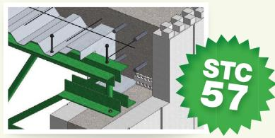
Ecospan is perfect for ICF wall framing systems (Insulated Concrete Forms)
