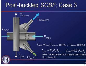
A Figure 2 (a and b). Determination of post-buckled SCBF connection forces from the "Where Did that Force Come From?" webinar.
